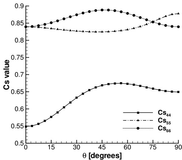
Figure 17: The variation of the diagonal components of the strain correction matrix  $\mathbf{C}_s$  representing the torsion and shear strain corrections. The results are shown for the angle-ply beam over a range of ply angles from  $\theta = 0^\circ$  to  $\theta = 90^\circ$ .
