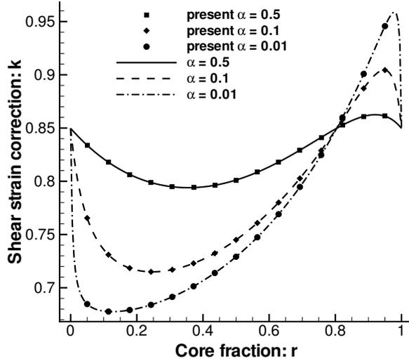
Figure 4: Comparison of the shear correction factor for the isotropic three layer beam. Finite-element results from the present approach are compared with Equation (46).
