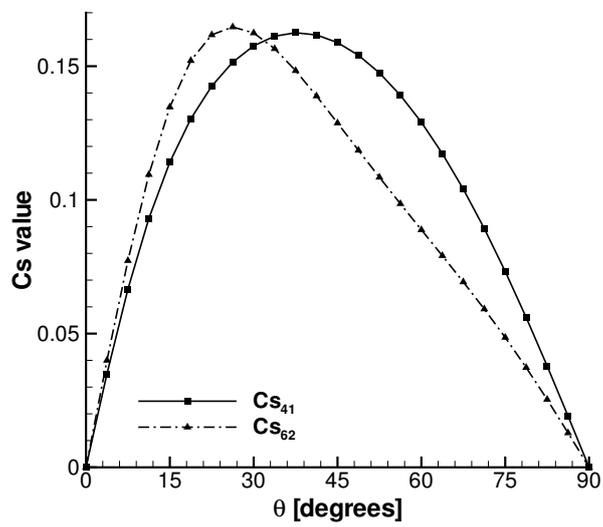
Figure 18: The variation of the off-diagonal components of the strain correction matrix  $C_s$ . The results are shown for the angle-ply beam over a range of ply angles from  $\theta = 0^\circ$  to  $\theta = 90^\circ$ .
