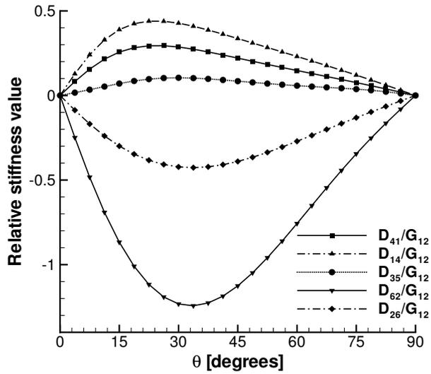
Figure 16: The variation of the off-diagonal components of the homogenized stiffness matrix  $\mathbf{D}$  normalized by the shear modulus  $G_{12}$ . The results are shown for the angle-ply beam over a range of ply angles from  $\theta = 0^\circ$  to  $\theta = 90^\circ$ .
