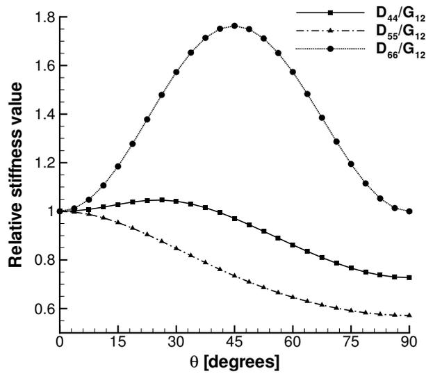
Figure 15: The variation of the diagonal components of the homogenized stiffness  $D$  representing the torsion,  $D_{44}$ , and shear stiffnesses,  $D_{55}$  and  $D_{66}$ , relative to the shear modulus  $G_{12}$ . The results are shown for the angle-ply beam over a range of ply angles from  $\theta = 0^\circ$  to  $\theta = 90^\circ$ .
