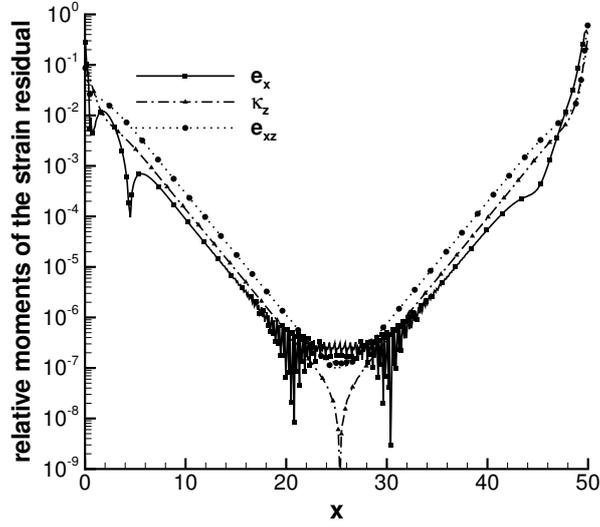
Figure 9: Components of the relative moments of the strain residual  $L_s \tilde{\epsilon}|_{3D}$  normalized by the maximum absolute values of the strain moment over the domain. These quantities are computed from a combination of the finite-element solution and the beam theory using Equation (48). These components are representative of the remaining components.
