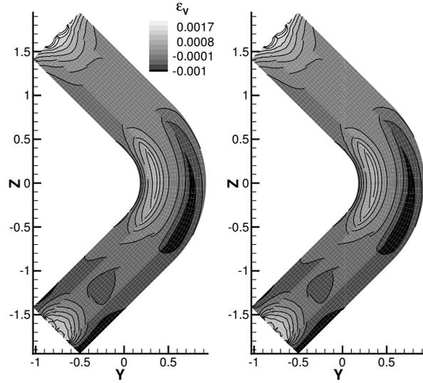
Figure 14: A comparison of the through-thickness volumetric strain  $\epsilon_V = \epsilon_x + \epsilon_y + \epsilon_z$  at the cross-section  $x = L/2$ . The beam theory solution is shown on the left, while the full three-dimensional solution is shown on the right.
