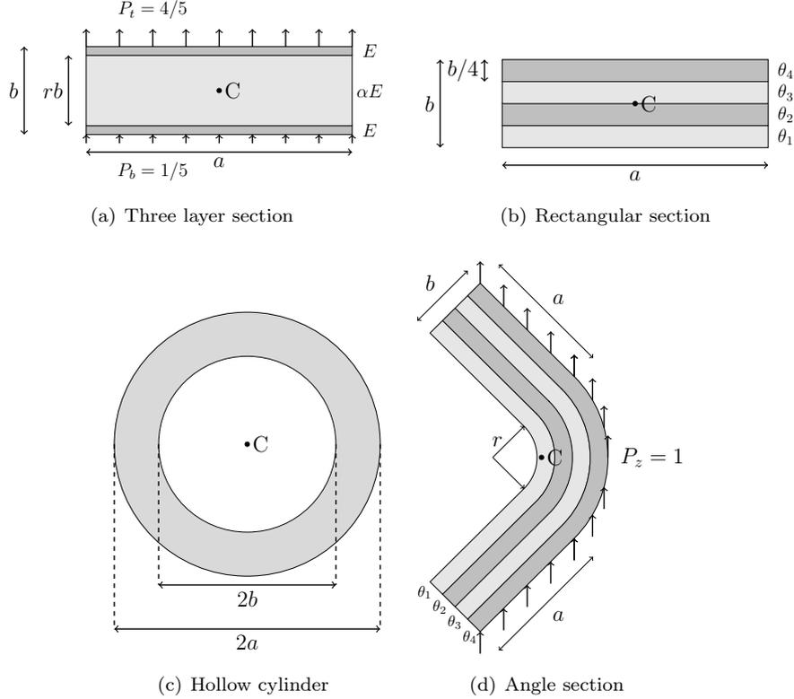
Figure 3: The section geometries used for comparison. The centroid of each section is marked with a C.
